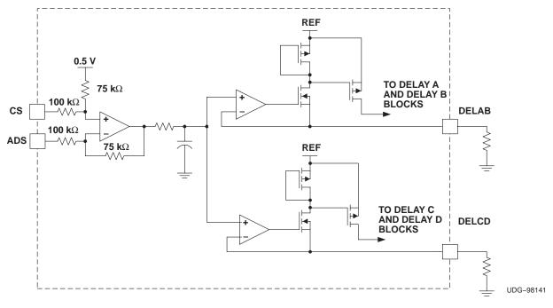
Figure 2. Adaptive Delay Set Block Diagram
