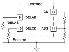
Figure 4. Programming Adaptive Delay Set
