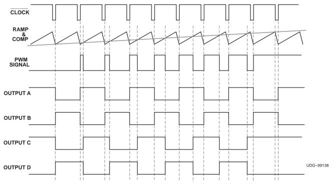
Figure 6. UCC3895 Timing Diagram (No Output Delay Shown, COMP to RAMP offset not included)
